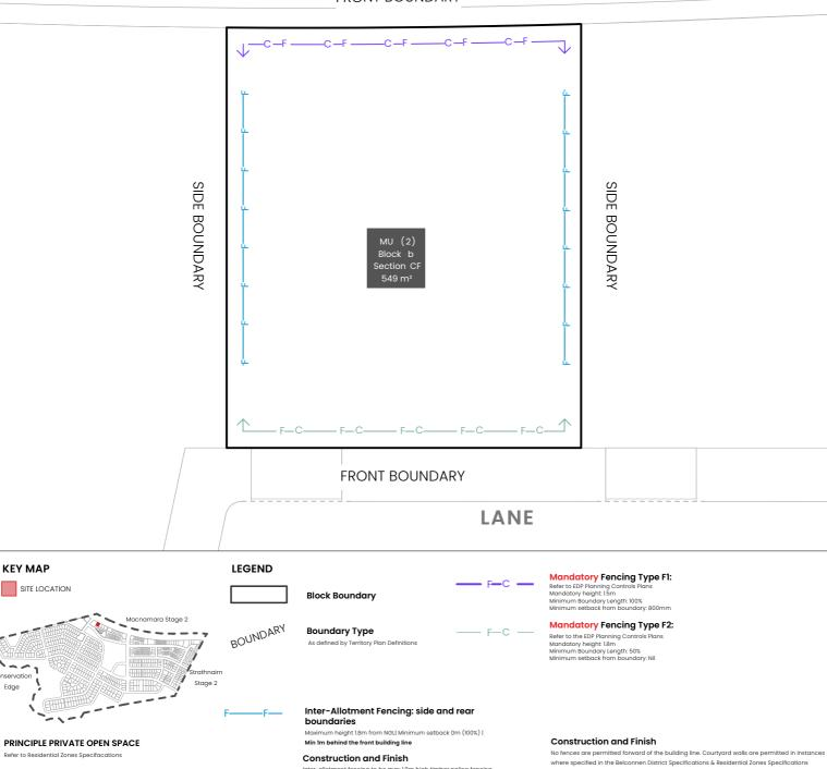
Inter-allotment fencing to be max 1.8m high timber paling fencing or lapped and capped timber paling fencing. If Colorbond is used, the profile must be Neetascreen or Miniscreen and colour "Jasper". Refer to Ginninderry Design Requirements (Macnamara)
