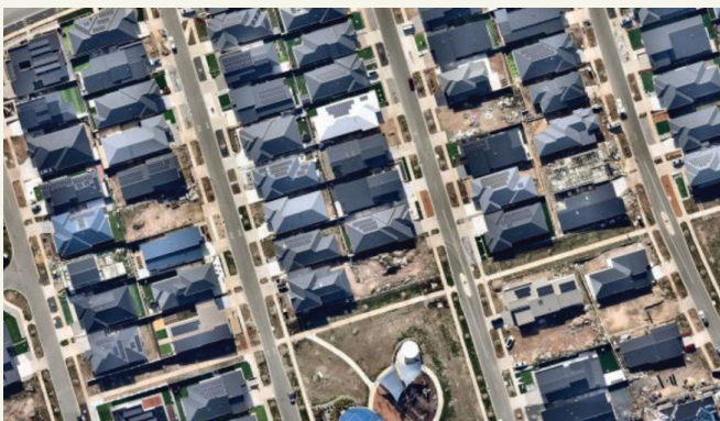
Darker roofs create excessive heat
