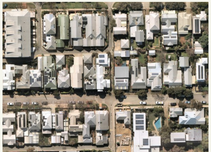
Lighter roofs reduce heat transfer
