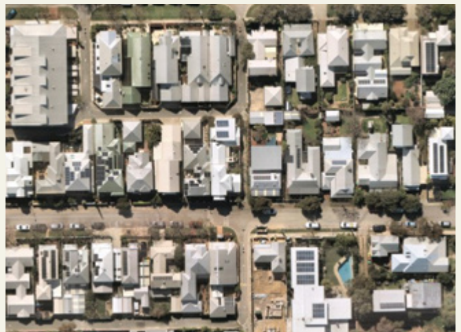
Lighter roofs reduce heat transfer
