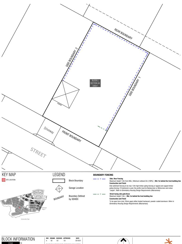
ZONE RZ3 SECTION AK BLOCK j CLASSIFICATION LARGE BLOCK HOUSING TYPE SINGLE DWELLING DO NOT SCALE OFF DRAWINGS. DIMENSIONS ARE IN METRET. INFORMATION ON THIS PLAN IS TO BE USED AS A MEUTRES. FOR THE DESIGN PROCESS APPROVED EDP PLANNING CONTROLS NEET DO BESS APPROVED EDP PLANNING ULTERS. PLANS TO BE READ IN CONJUNCTION WITH THE TERRITORY PLAN ALONG WITH BLOCK DISCLOSURE PLANS AND THE GININDERRY DESIGN REQUIREMENTS O CONFIRM ALL CURRENT CONTROLS PERTAINING TO YOUR BLOCK.
