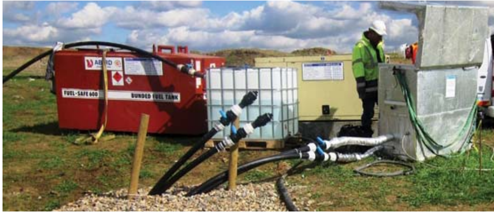
Figure 8 A mobile thermal response testing unit connected to a buried ground collector loop.
