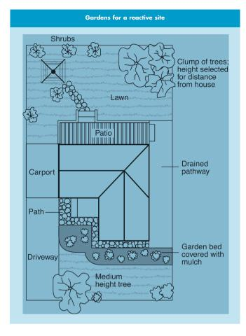
extend outwards a minimum of 900 mm (more in highly reactive soil) and should have a minimum fall away from the building of 1:60. The finished paving should be no less than 100 mm below brick yent bases.
