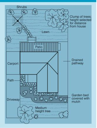
extend outwards a minimum of 900 mm (more in highly reactive soil) and should have a minimum fall away from the building of 1:60. The finished paving should be no less than 100 mm below brick vent bases.
