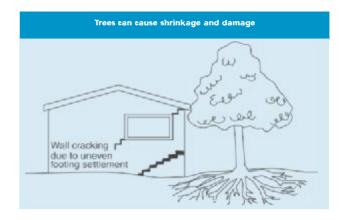
As the weather pattern changes and the soil begins to dry out, the external footings will be first affected, beginning with the locations where the sun's effect is strongest. This has the effect of lowering the external footings. The doming is accentuated and cracking reduces or disappears where it occurred because of dishing, but other cracks open up. The roof lines may become convex.
