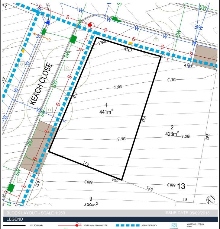
STORMWATER MAIN / SUMP / FASEMENT NRNCo PIT SUBSTATION MANHOLE / TIE WATER MAIN / STOP VALVE / HYDRANT / TIE 550.0-CONTOUR 0.5m INTERVAL STREETLIGHT STREET TREES CONTOUR 0.1m INTERVAL WATER MAIN (IRRIGATION) ABOVE GROUND MINIPILLAR REINFORCED CONCRETE DRIVEWAY BY PURCHASER GARAGE OFFSET FROM REAR BOUNDARY (1.0) IN GROUND MINIPILLAR MANDATORY TWO(2) STOREYS FRONT FENCING AND GATE BY DEVELOPER BLOCK SUBJECT TO MID-SIZED PROVISIONS POTENTIALLY NOISE AFFECTED BLOCK ACCESS ROUTE REQUIRED
